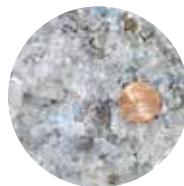
PET Flake w/Aluminum (<4mm) 93% Aluminum Contamination Removed
