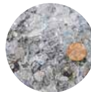
PET Flake w/Aluminum (4mm-10mm) 96% Aluminum Contamination Removed
