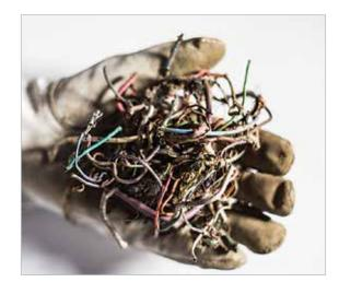
ICW Wire Magnetically pulling stainless out of dirty streams to remove wire before chopping line
