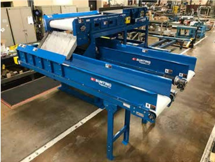
Note: Generally 2” minus fractions work great on 4” diameter HISC™ Pulleys while larger 4” minus fractions need the 6” diameter HISC™ Pulleys.
